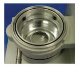
If gasket does not move freely, remove it and clean with a small amount of liquid dish soap applied and removed with a dry paper towel. Lubricate pins and springs and replace gasket.
