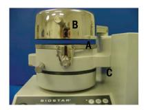
The heating surface (A) should be parallel to the heating element (B). Adjust the position of the chamber by turning the screw (C), located under the chamber support frame on the side of the unit, with a screwdriver. Counter-clockwise adjustment elevates the chamber.
