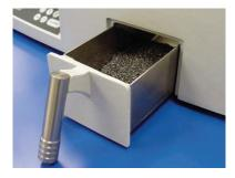
Pellets will become dirty with regular use. Clean pellets by placing them in a strainer and rinsing with hot water. Spread pellets on a towel and let air dry before placing them back in the Biostar. Check pellets monthly, discard and replace pellets in the bottom third of the cup.
