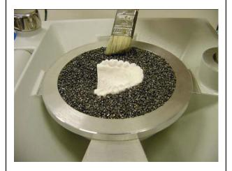
Remove the pellet drawer and pour pellets between the model and the inner wall of the cup. Apply more than enough pellets in these areas. Use a Biostar brush to remove excess pellets and level the pellet line from the occlusal-incisal plane to the top rim of the cup. Hold the brush at an angle to sweep excess pellets from the rim of the cup and the palatal area of the model.
