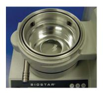
Clean and lubricate gaskets every 3 months. Apply a drop of liquid dish soap onto the gasket on the pressure chamber with a fingertip. Identify potential gasket cuts or irregularities. Remove the soap from the gasket with a soft cloth.
