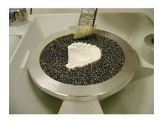
Make sure all pellets are removed from edge of cup where the chamber locks into place. Pellets should be even with top of pellet cup.
