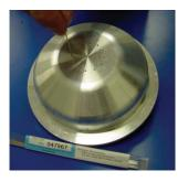
Air escape holes are present in the base of the pellet cup and should be checked monthly to ensure that they remain open. Use a .036" or thinner diameter wire to open plugged holes. Also, make sure the rim of the pellet cup and the four blocks that support the cup are clean.
