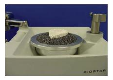
For mounted models, remove the majority of pellets. Leave only enough under the model to allow air to flow. Build up the pellets, leaving exposed only the area to be covered by acrylic material.
