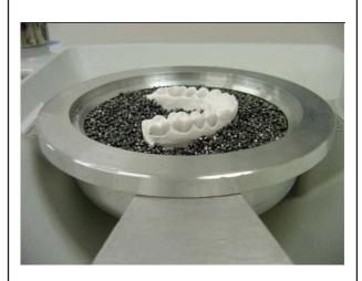
For example, when constructing an orthodontic retainer, the pellets are placed against the occlusal-incisal margin to cover the wax holding the wires facially. The pellets act as an insulator when the heated material is formed.
