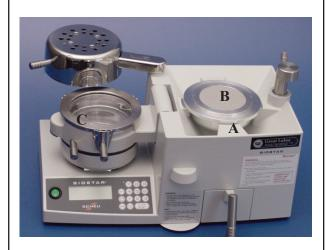
**A – Platform:** Circular plate that is placed on the inner lip of the pellet cup.
