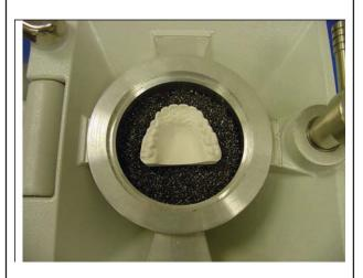
Enough pellets must be placed in pellet cup to hold the model at proper level. Material termination areas, located on the facial surface of the model, should be referenced at the same height as the top ledge of the pellet cup.
