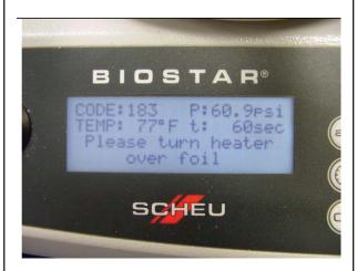
**CODE:** Three-digit code to identify heating and pressure molding times.
