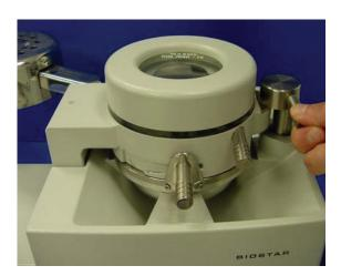
At this point in the process, the material has been formed over the model and is cooling under pressure.
