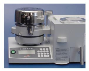
To initiate heating, swing the heating element over the clamped material and the programmed time will start to count down automatically. With five seconds remaining in the heating phase, a series of short beeps will sound, at zero, a sustained beep will sound.
