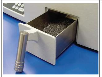
Pellets will become dirty with regular use. Clean pellets by placing them in a strainer and rinsing with hot water. Spread pellets on a towel and let air dry before placing them back in the Biostar. Check pellets monthly, discard and replace pellets in the bottom third of the cup
