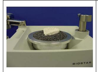
Models mounted to articulator plates should be splitcast. If the model cannot be removed from the mounting, the pellet level will need to be at a slight incline; to appliance termination areas.
