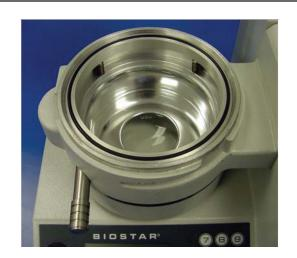
Clean and lubricate top gasket every 3 months. Apply a drop of liquid dish soap onto the gasket on the pressure chamber with a fingertip. Identify potential gasket cuts or irregularities. Remove the soap from the gasket with a soft cloth.
