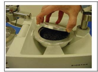
Place the pellet cup flush onto the four metal blocks on the Biostar table. Empty cup or reduce the pellet line to the half-way level. Make sure the inner lip of the cup is clean. Place the outer ring of the platform on the inner lip of the pellet cup with the flat platform surface on top.
