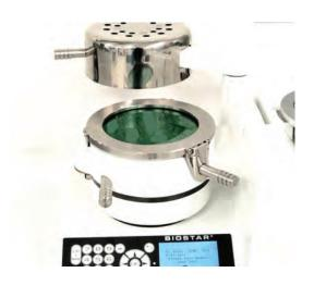
Align the clamping frame over the material so that the three clips slip under the bevel of the locking device on the sides of the chamber.
