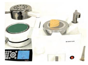
Position the model on the platform, referencing the heel toward the material in the pressure chamber, and incisor segment near the center area of the platform. Placing the model to the left side of the platform provides better material forming along the incisor region.
