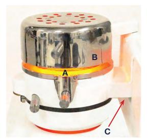
The heating surface (A) should be parallel to the heating element (B). Adjust the position of the chamber by turning the screw (C) located under the chamber support frame with a small screwdriver.
