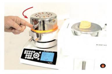
Swing the heating element from its rest position over the material (curved red arrow) on the pressure chamber. When the heater is placed over the material, the heating element illuminates and the set heating time begins.
