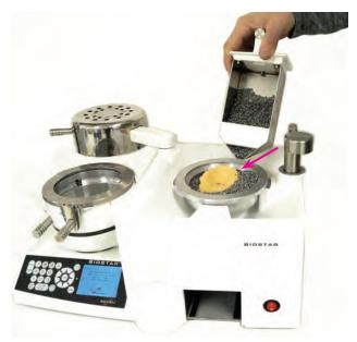
Pour pellets between the model and the inner wall of the cup (red arrow). Apply additional pellets in this area as needed.
