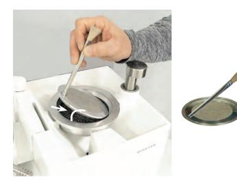
Empty cup or reduce the pellet line to the half-way level (white arrow). Make sure the inner lip of the cup is clean. Place the outer ring of the platform on the inner lip of the pellet cup with the flat platform surface on top (curved white line).
