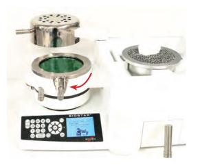
Tighten by turning the handle clockwise, so that the chamber and clamping handles are parallel (curved red arrow). Note: To ensure a tight seal between the pressure chamber and the cup, pellets should be completely removed from around the rim.
