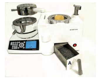
Remove the pellet drawer (A) from the machine by pulling the drawer out using the handle.
