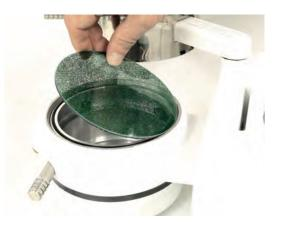
Position a 125mm diameter round disc on the spring-loaded adjusting ring of the pressure chamber.
