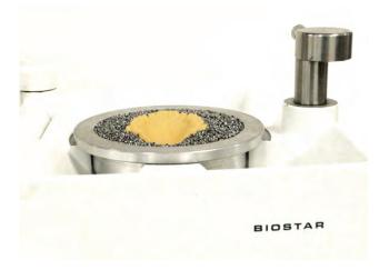
Place an adequate amount of pellets in the pellet cup to elevate the model at the proper level. Material termination areas, located on the facial surface of the model, should be referenced at the same height as the top ledge of the pellet cup.
