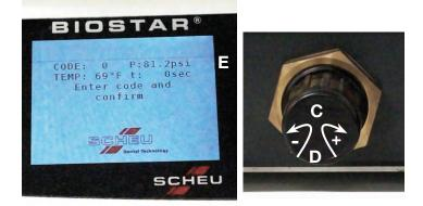
8. Working pressure of 87psi is pre-set in the machine. With the power button in the 'ON' position, press the CODE/SCAN button (A). The current pressure will show on the LCD display. Confirm or adjust the Biostar air pressure (B) if needed. Suggested operating pressure is 80psi
