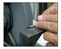
The Carbon Soldering Tip (240-061) should be ground, filed, or sanded to a point at one end of the rod. This may have to be repeated as flux builds up on the pointed end of the Carbon Tip.
