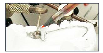
Hold the Carbon Tip against the solder ball and metal on the model until desired solder flow is accomplished. The Carbon Tip will heat-up and glow **red** during this procedure. To conclude the process, move the model from the electrode wire in the Auxiliary Plug-in Vise and Carbon Tip.
