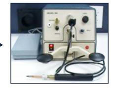
Adjust the welder dial on upper left side of the front of the machine to a 1 or 2 setting. The higher the setting, the quicker the metal parts being soldered will heat. Do Not overheat metals during this process. Press down the swing arm with the two black circular pads and lock in this position with the lock lever (L). This turns on the soldering feature of the welder.
