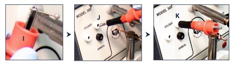
The Alligator Clip of the Auxiliary Plug-in Vise is squeezed to open the clip part (I). Insert the wire end of the soldered electrode (S, M, L, XL) into the open end of the Alligator Clip. Place the plug end of the Auxiliary Plug-in Vise into the top, right white plug (J), with solder electrode pointing to the left side of Spot Welder (K).
