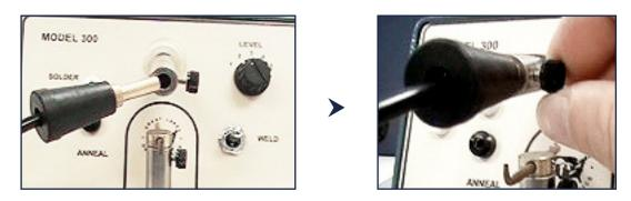
Insert the plug end of the Auxiliary Cable into the top plug where the electrode was removed. Tighten the thumb screw to secure the plug end of the cable to the welder.
