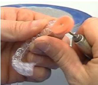
18 A miniature satin buff or coarse Dymo wheel is used with a lab handpiece to smooth trimmed edges.
