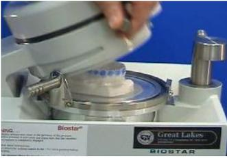
13 Swing the chamber open and remove the formed material from the platform.
