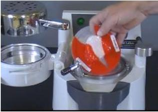
13 At the end of the cooling cycle, release the pressure, unlock the chamber and open the machine. Remove material and model from platform.
