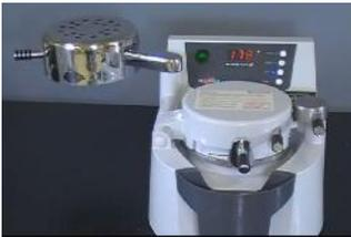
12 At the end of the heating cycle, remove the heater and swing the chamber over the model on the platform. Lock chamber in place to initiate the forming and cooling cycle. Allow formed material to cool under pressure for 3-5 minutes.
