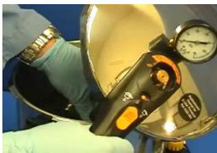
5 Place the model and acrylic resin into a humid pressure pot for 15 minutes. Pressure should be adjusted to approximately 20psi. At the end of the curing cycle, evacuate the pressure and remove model and cured acrylic.
