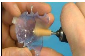
18 A sandpaper mandrel with a 3" piece of 150-grit sandpaper is used with a lab handpiece on medium speed to smooth trimmed surfaces.
