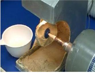
25 A rag wheel is moistened and attached to a dental lathe using low speed. Then water is mixed with a medium grade pumice.
