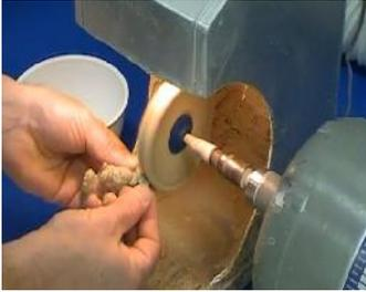
26 Apply pumice to the plastic teeth and press against wheel. Smooth acrylic surfaces, add additional pumice as needed. Rinse and dry plastic teeth.
