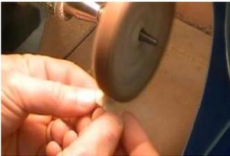
28 Apply Tripoli polish to the wheel. This polish is used to remove fine scratches that the pumice agent may have incorporated. Polish plastic teeth. Remove the wheel with Tripoli polish and replace it with a second 4 inch muslin buff wheel.
