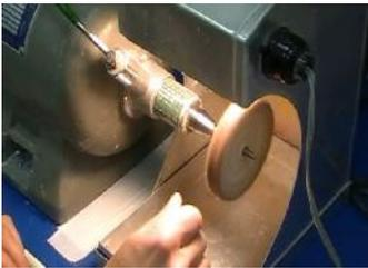
27 Turn on lathe to low speed. Attach a 4 inch muslin buff wheel to the quick chuck mechanism on the lathe.
