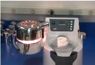
4 Place a sheet of 2mm or 3mm thick mouthguard or Bioplast material on the pressure chamber. Secure in place with the clamping frame. Input code 183 (60 seconds heating) for 2mm thick material or 233 (90 seconds heating) for 3mm thick material. Position the heater over the clamped material to start the heating cycle.
