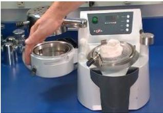
6 Once the pressure molding cycle has concluded, evacuate the air pressure from the chamber and unlock the chamber with the handle on the right side (12 o'clock position) of the machine. Slide the clamping frame to the left to release the formed material from the pressure chamber. Open the pressure chamber.
