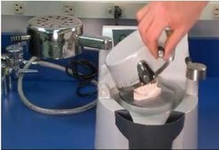
5 Once the heating cycle is complete, remove the lamp and swing the pressure chamber over the model on the platform. Lock the chamber in place by rotating the handle on the right side of the machine from the 12 o'clock position to a 6 o'clock position. Cool formed material under pressure for 120 seconds.
