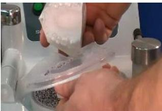
7 Remove the model with formed material from the platform. Pull the opposite corners to release the material from the model. Holding the model base, carefully pull the model from the mold without turning the mold inside out.
