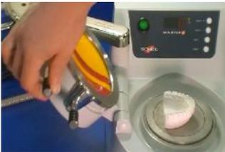
9 Once the second heating cycle is complete, remove the lamp and swing the chamber over the model on the platform and lock in place to initiate forming phase. Allow the material to cool under pressure for 2-3 minutes.
