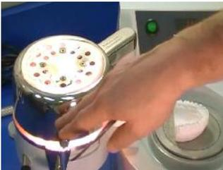
8 Enter 15 seconds into the machine and swing the lamp over the material to initiate the second heating stage.
