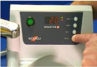
6 For this application, the pressure should be reduced to 2 or 2 ½ bar or 30 psi. Adjust pressure below desired level, then increase. Higher pressure could cause strips to separate as they are formed. Heating time will be increased to compensate for the use of lower pressure. The heating cycle will be accomplished in two stages. First, enter 90 seconds of heating time for the initial stage. Later, a 15 second stage will be entered. Swing the lamp over the chamber to initiate the heating cycle.
