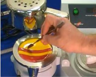
7 At the end of the first heating cycle, remove the lamp and seal the strips together with a wax spatula.
