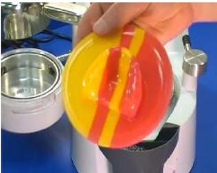
10 After forming and cooling cycle are complete, evacuate pressure and open chamber. Remove the formed material and model from machine.
