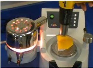
6 Turn the heat gun on high and swing the heated lamp over the clamped material to start the heating cycle. With about 50 seconds remaining in the heating cycle, soften the template lying on the model with the heat gun. As the heating cycle nears its conclusion, material over the model should drape around the model. A decal or patient name can be placed on the colored material along the incisal region.
