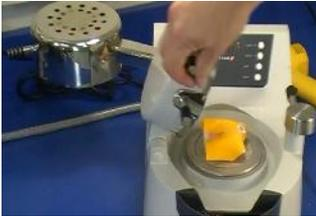
7 At the end of the timed heating cycle, remove the lamp from the material and swing the chamber over the model on the platform. Engage the locking handle to start the molding and cooling process. The formed material should be under pressure for 2 to 2 ½ minutes.
