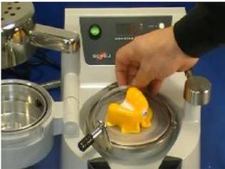
8 Evacuate the pressure from the chamber at the end of this cycle. Unlock the chamber and clamped material. Swing open the chamber and remove the formed material and model from the platform.
